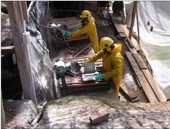
PHOTO 10-1: CUTTING CORE WITH A DIAMOND SAW
